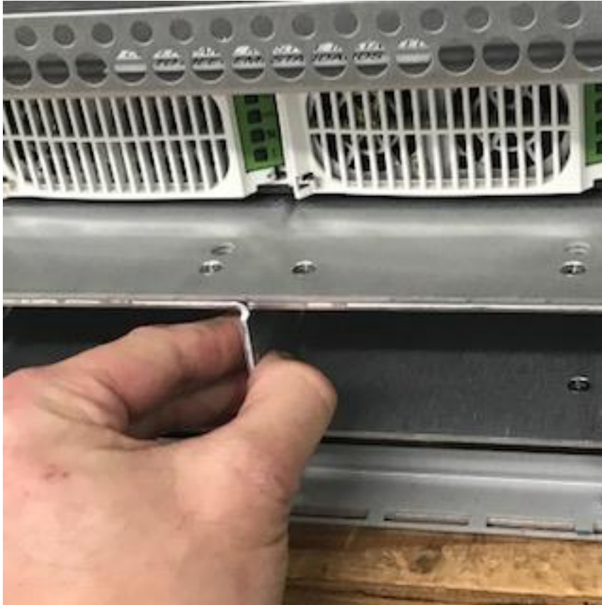
Figure 12 Removing PS tray
