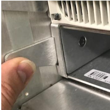
Figure 11 left side release
