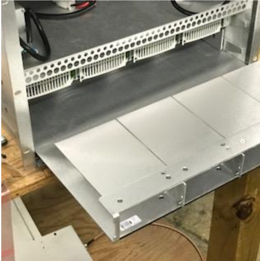
Figure 13 Half way out, Keep it straight
