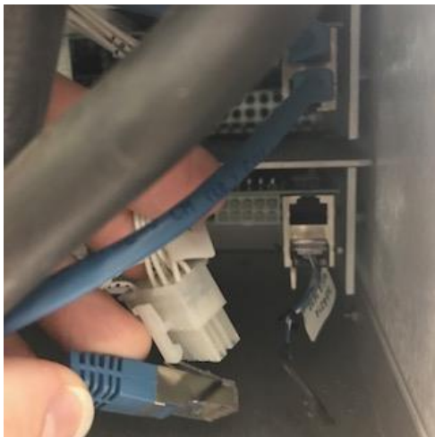
Figure 2 disconnection of J1 & J3
