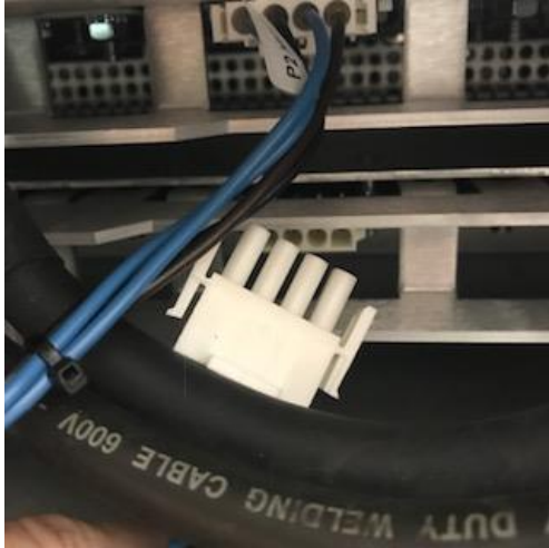
Figure 3 disconnection of J2
