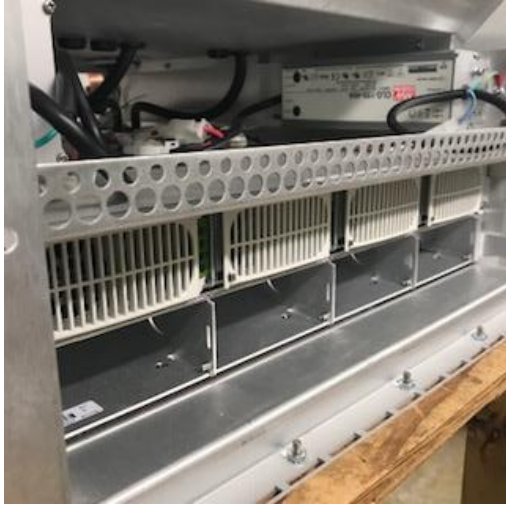
Figure 7 PS 5 through 8 removed
