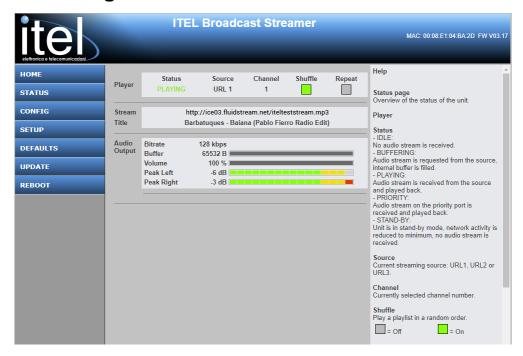
The module adds audio streaming decoding capabilities for receiving streaming MP3 / AAC + shoutcast servers or by using RTP and TCP / IP connectivity. The module also allows playback of audio files from an USB key.
