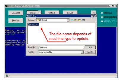
7. Wait until the end of programming. Verify that the operation is successful. In case of failure, shut down the machine, close the program, wait a few seconds, repeat the above steps related to programming. In case of success, turn off the machine, close the program, reposition the switch under the grid on "Run Mode".
