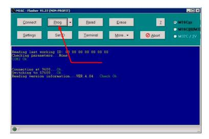
6. As soon as the link between machine and P.C. it was established should be inserted path and file name with which to program the flash memory of the microprocessor. Click on "Open" or press ENTER to start planning.
