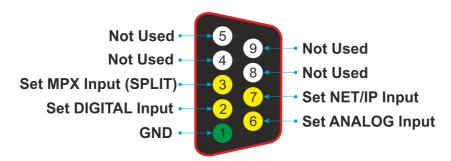
The inputs are activated by grounding the relative pin or by providing a voltage from 5 to 12VDC, in this case the jumpers placed on the board inside the device will have to be moved from the "CLOSE" to "VIN" position.
