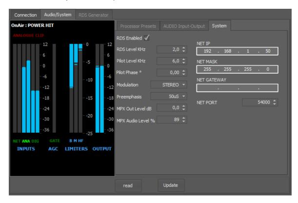
The network parameters are related to the optional network module only. If the streaming module was installed, network configuration will be done through the web server of the module.
