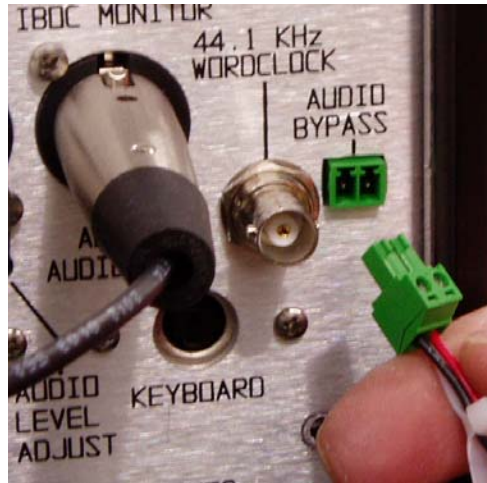
Figure 11 – Disconnect AUDIO BYPASS Cable
