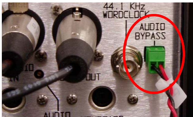
Figure 38 – Connect the AUDIO BYPASS Cable
