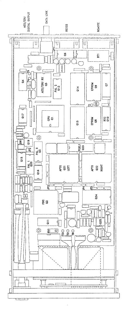
DISC TRAK DC-10 MECHANICAL DETAIL BOTTOM ELEVATION - PROCESSOR BOARD
