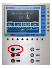
Figure 18 - Turn the RF Output Power ON
