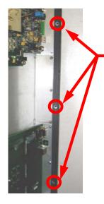
**Step 2** – Using a No. 2 Phillips Screw Driver remove the (3) screws from the hinge area as shown
