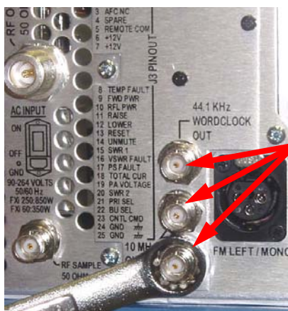
Figure 18 – Install BNC Connector Hardware
