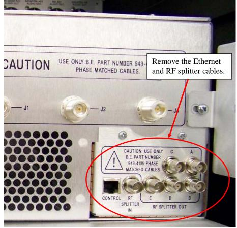
Figure 6. Remove Ethernet and BNC cables.
