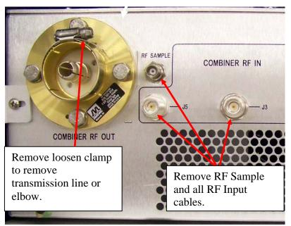
Figure 5. Remove transmission line and RF cables
