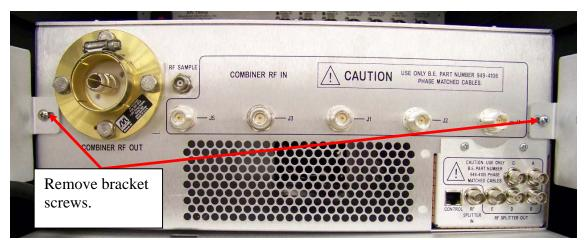
Figure 7. Remove bracket screws.
