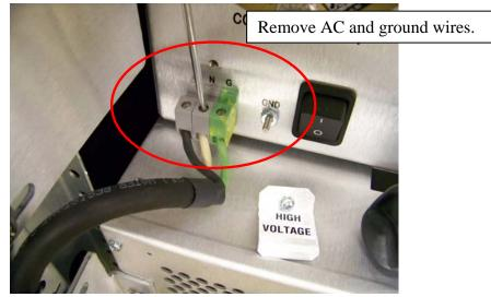
Figure 2. Remove wiring
