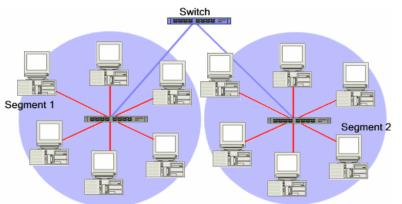
A switch is a network device that separates multiple segments on a network, but is smart enough to know if a particular packet needs to be sent to the other side.
