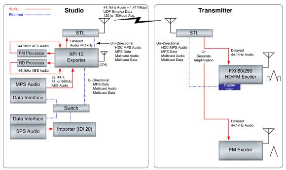
connection to the transmitter site. This is the only architecture allowing you to send HD Radio data to the transmitter site over a simplex (unidirectional) UDP connection.
