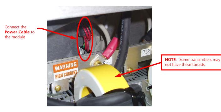
Figure 11 – Connect Power Cable
