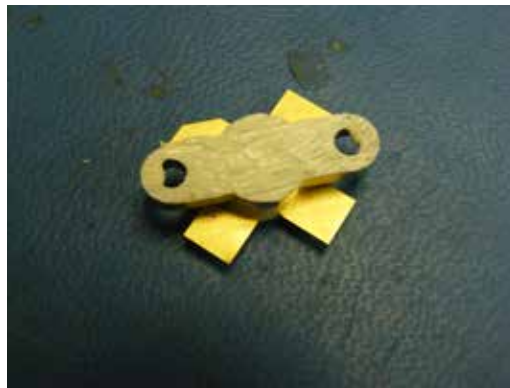
Figure 98 – Driver with Thermal Compound Applied
