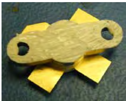
Figure 100 - Bottom of RF Power Amplifier with Grease
