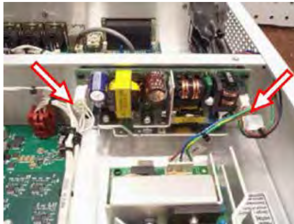
Figure 67 - Fan Power Supply Cable Removal
