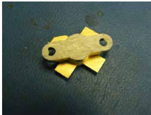
Figure 111 – Driver with Thermal Compound Applied
