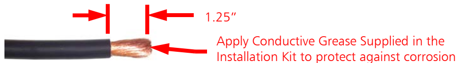
Figure 22 – Suggested Strip Length and Grease for AC Supply Wiring
