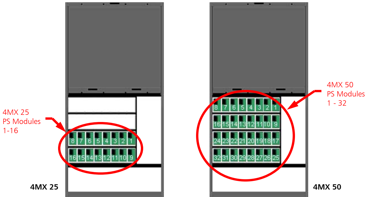
Figure 172 – Power Supply Module Locations (Rear of Transmitter)
