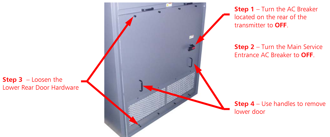
Figure 180 – Turn the Transmitter's AC Breaker OFF and Remove Door
