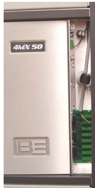
Figure 116 – Remote Control I/O Access Panel Removal
