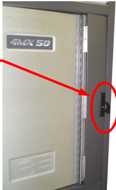
Figure 93 – Remote Control I/O Access Panel Removal
