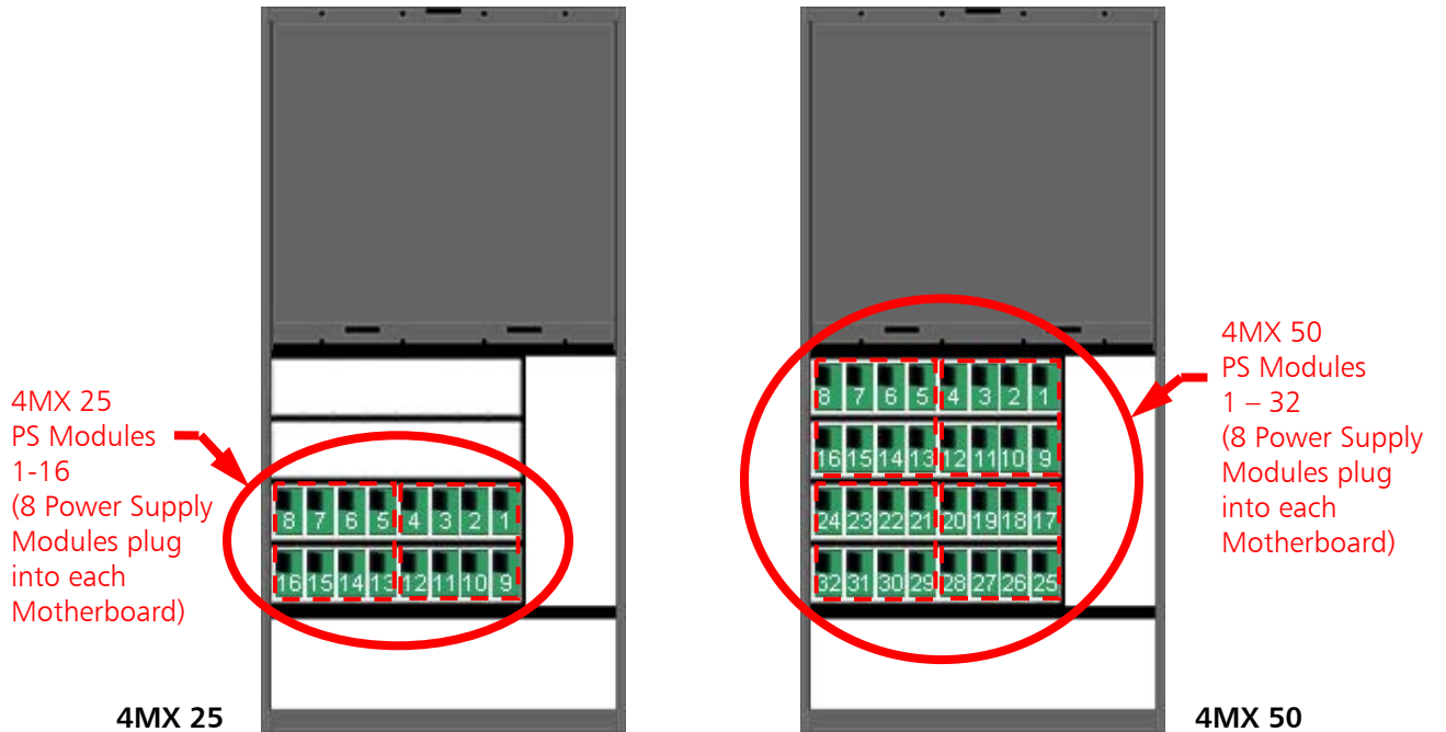
Figure 181 – Power Supply Module Locations (Rear of Transmitter)
