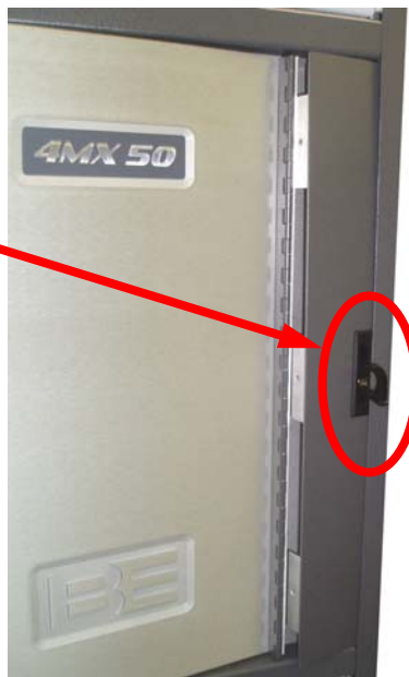
Figure 211 – Remote Control I/O Access Panel Removal
