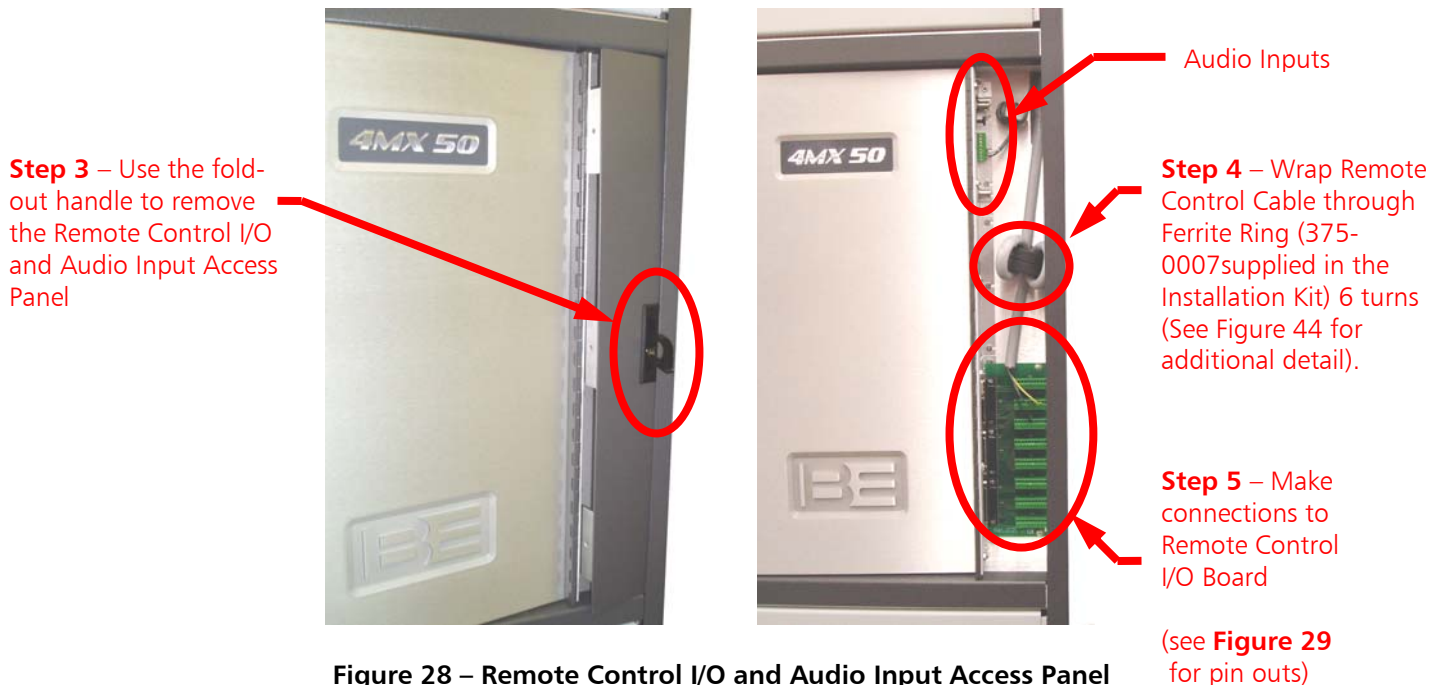
Figure 27 – Remote Control I/O and Audio Input Access Panel Hardware
