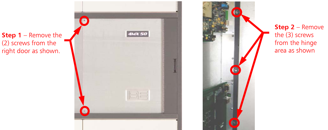
Figure 77 – Remote Control I/O and Audio Input Access Panel Hardware
