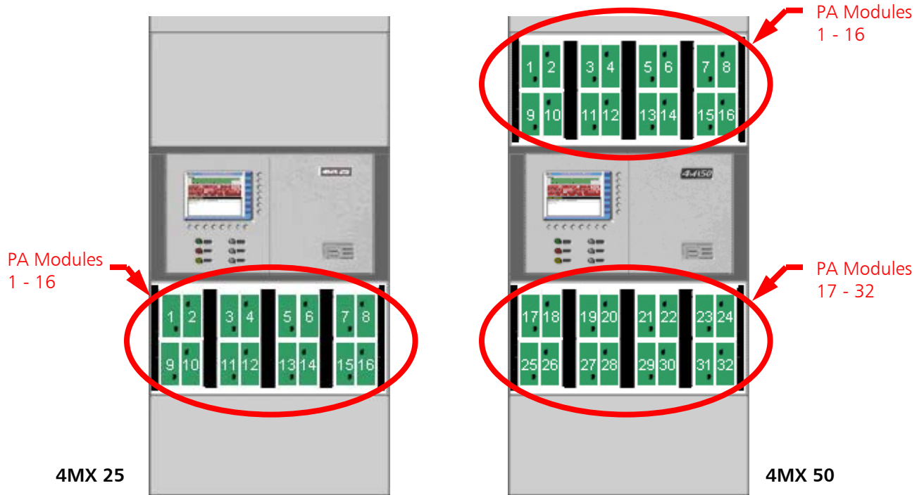
Figure 134 – PA Module Locations (Front of Transmitter)
