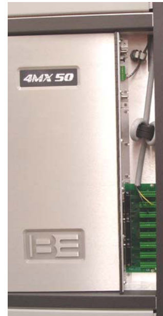
Figure 193 – Remote Control I/O Access Panel Removal
