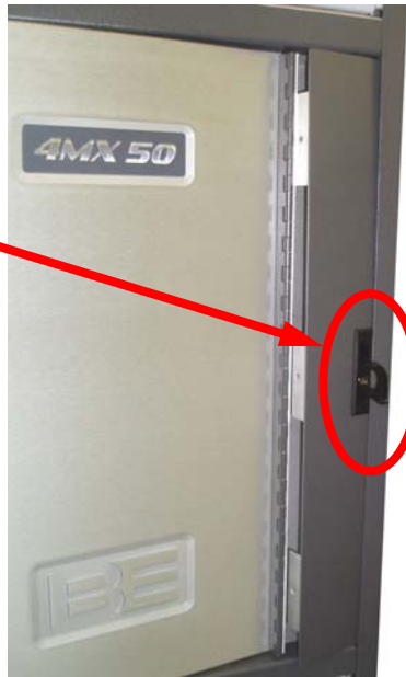
Figure 193 – Remote Control I/O Access Panel Removal
