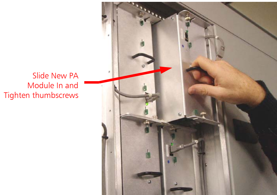
Figure 138 – Install New PA Module and Tighten Thumbscrews
