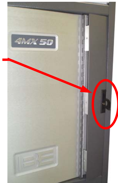
Figure 116 – Remote Control I/O Access Panel Removal
