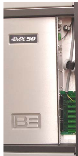
Figure 211 – Remote Control I/O Access Panel Removal
