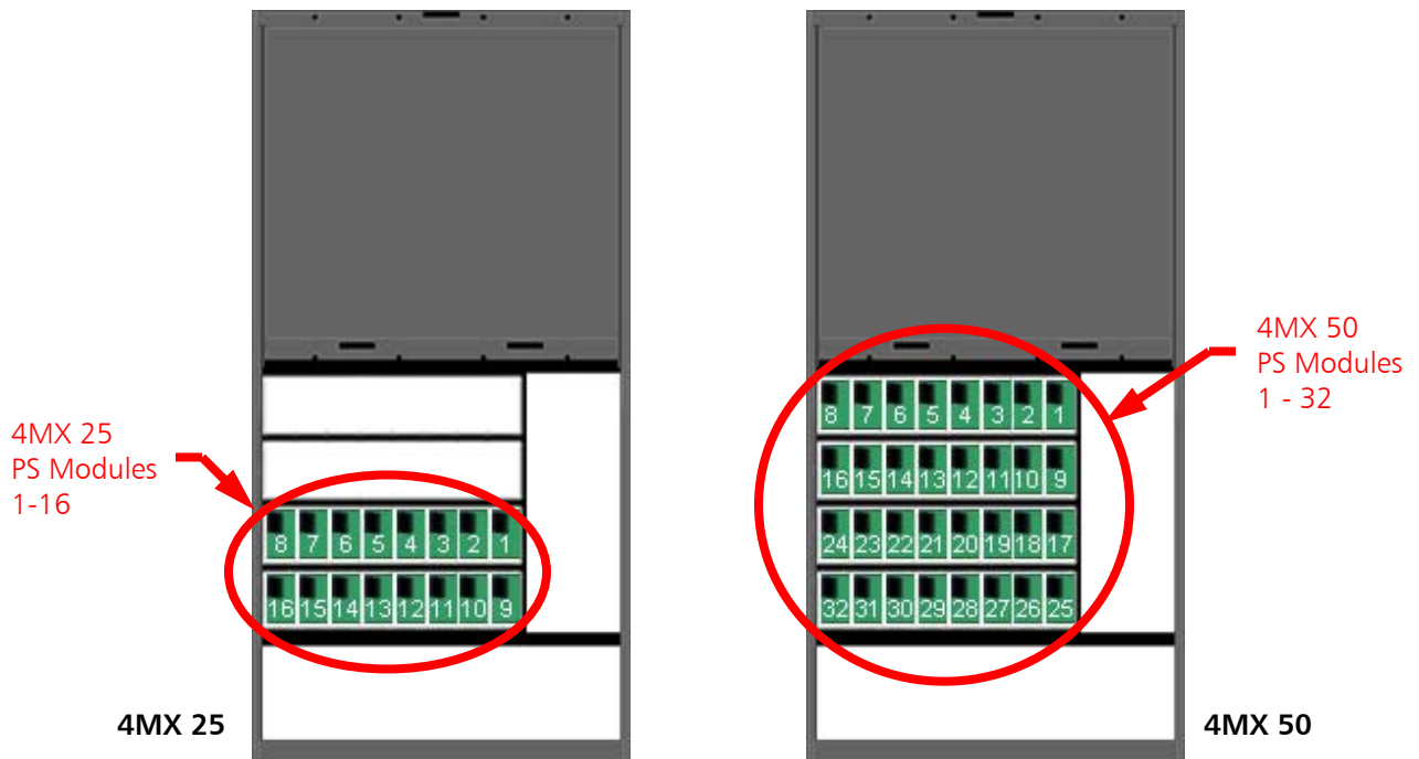
Figure 168 – Power Supply Module Location (Rear of Transmitter)
