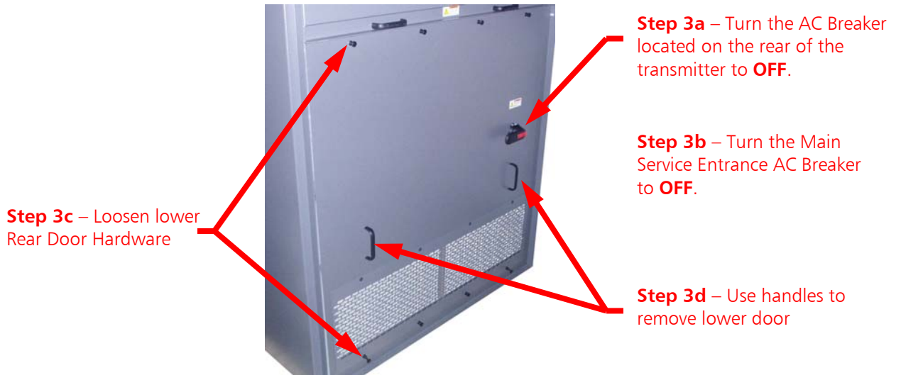
Figure 171 – Turn the Transmitter's AC Breaker OFF and Remove Door
