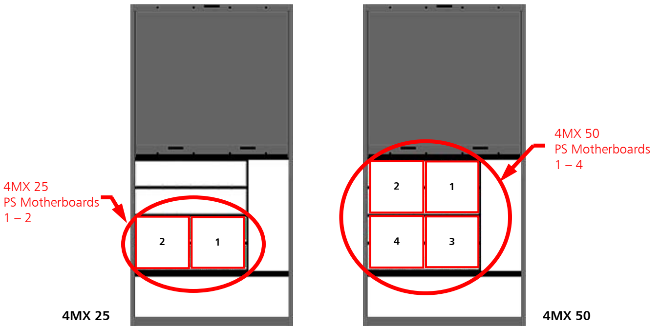
Figure 182 – Power Supply Motherboard Locations (Rear of Transmitter)
