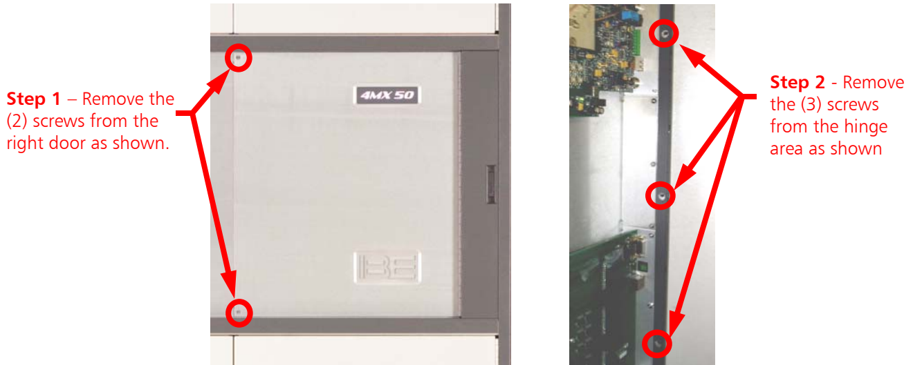
Figure 27 – Remote Control I/O and Audio Input Access Panel Hardware
