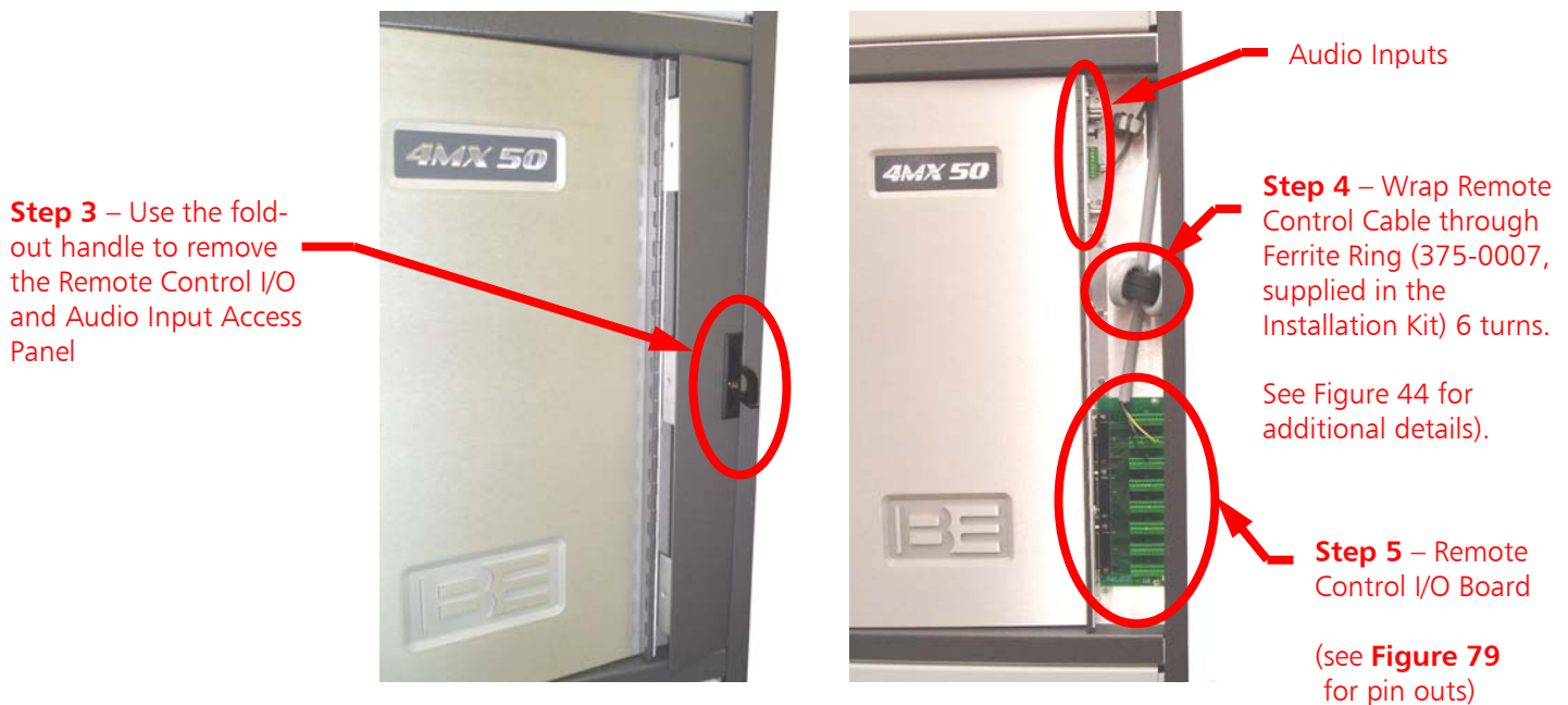
Figure 78 – Remote Control I/O and Audio Input Access Panel
