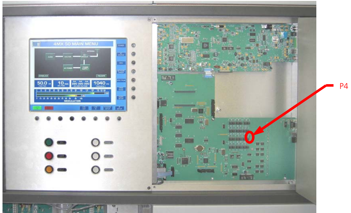
Figure 30 – Controller Board I/O Signal Configuration Jumper
