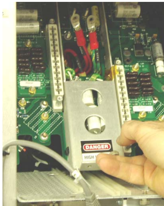
Figure 159 – Tilt Motherboard into Vertical Position
