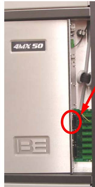
Figure 93 – Remote Control I/O Access Panel Removal
