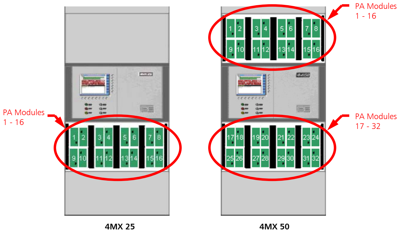
Figure 131 – PA Module Locations (Front of Transmitter)
