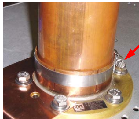
Figure 11 – 3-1/8 Inch, 50 Ohm, RF Output Connection
