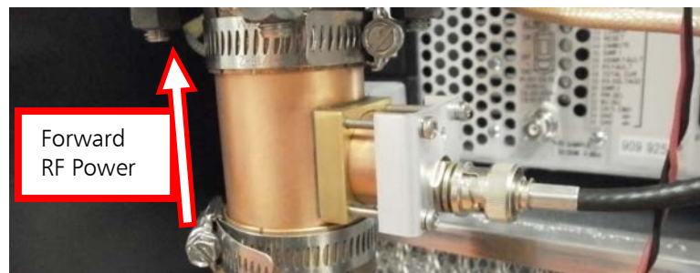
Figure 43 – 1 5/8" RF Coupler Detail
