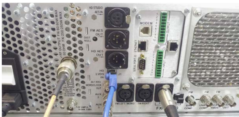
Figure 27 – IBOC System with VPe and Engine Ethernet & I/O
