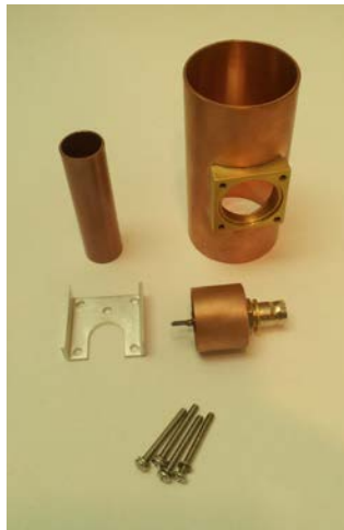
Figure 35 – RF Sample Coupler Parts
