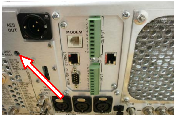
Figure 34 – Distortion Null Pot
