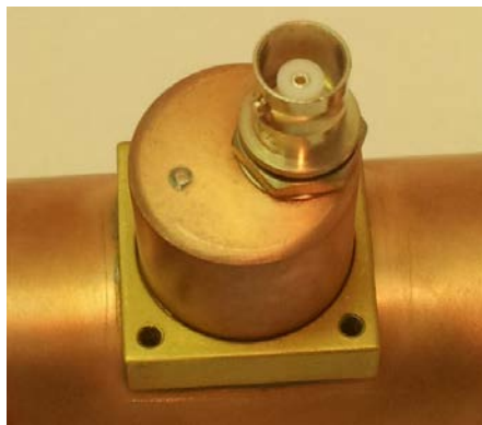
Figure 36 – RF Sample Coupler Assembly Step 1
