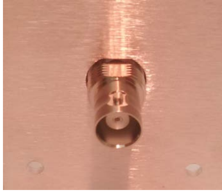
Figure 51 – Bulkhead BNC in Panel D Hole
