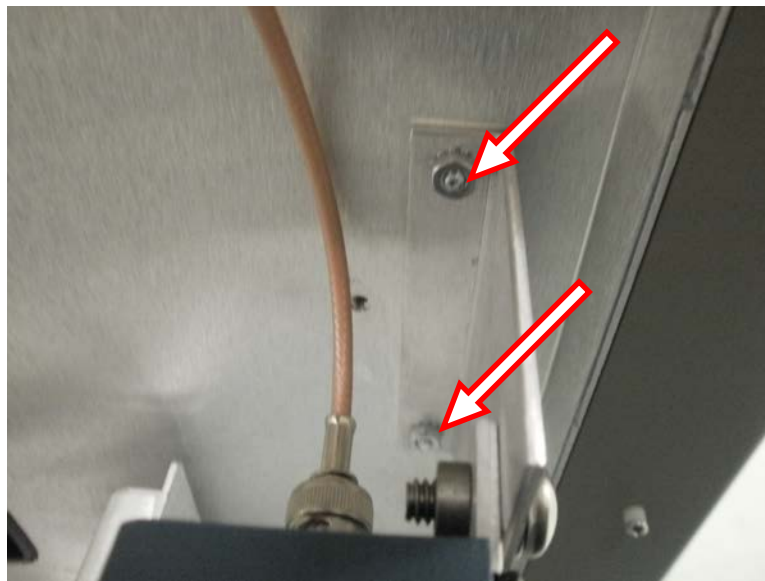
Figure 57 – FMi 301 and 402 Attenuator Mounting Bracket
